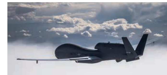
A NATO RQ-4D Phoenix remotely piloted aircraft during a mission; The High-Altitude Long-Endurance aircraft usually operate at a flight level above 50,000 feet – well above civilian air traffic. Archive photo courtesy NATO ISR Force
