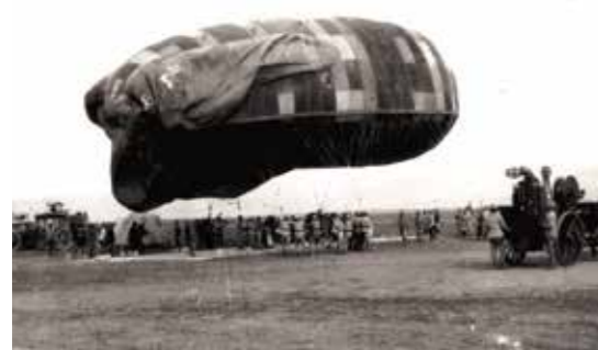
Preparing a Caquot aerostat for take-off. These aerostats had a good stability when ascending, even if the wind was over 70 km/h. Having only one observer in the nacelle, it could climb up to 1,800 meters, and up to 1,200 meters with two observers. As the photo shows, the nacelle could hold up to three people. The control cable was 7 mm thick and resisted to 3.6 tons.
