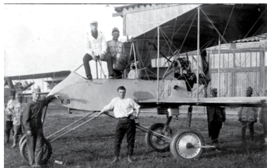
The Voisin III airplane, 130 Hp, in the Băneasa aeronautical center: imported from France in the autumn of 1915, it proved to be an excellent airplane for the missions of the air observers.
