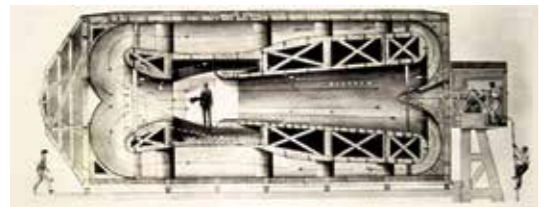
The Stroescu wind tunnel built at the Polytechnical School in Bucharest. in Bucharest
