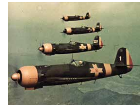
The most important product of the Romanian aeronautical industry was, for the first half of the 20 th century, the fighter IAR-80 manufactured by IAR Brașov. The engineers Ion Grossu and Ion Coșereanu were the leaders of the team that designed the IAR-80. It was an entirely metallic aircraft, with retractable landing gear and with a three-blade propeller which was 3 meters in diameter and had a variable pace. The prototype, which appeared in 1940, reached 510 km/h, which ranked it fourth in the world when it came to speed. The test extended up to 1940, when the ratification commission concluded that the plane "was a good interceptor due to its climb speed. It doesn't have any piloting-related flaws making it accessible to any well-trained fighter pilot having training related to avionics." It went into mass production in September 1940, and until the end of World War II approximately 5,000 aircraft were manufactured.
