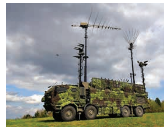
The primary jamming platforms utilized in this year's Ramstein Guard exercise included the Dassault Falcon 20 aircraft (right) operated by the British civil contractor Draken Europe and the cutting-edge STARKOM mobile communication jammer mounted on the Tatra Force 8x8 chassis (left), employed by the Opava 532 nd Electronic Warfare Battalion. Photo: 212 th Tactical Squadron and Army of the Czech Republic
