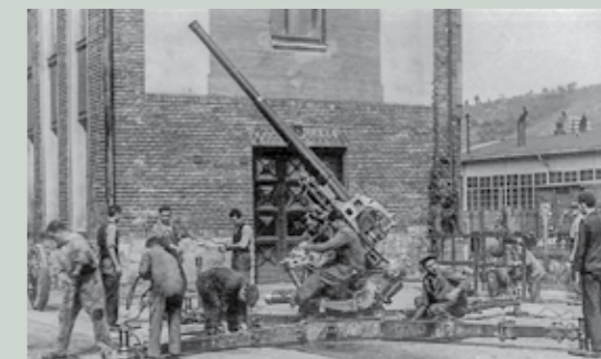
Mounting of an anti-aircraft artillery piece, caliber 75 mm
