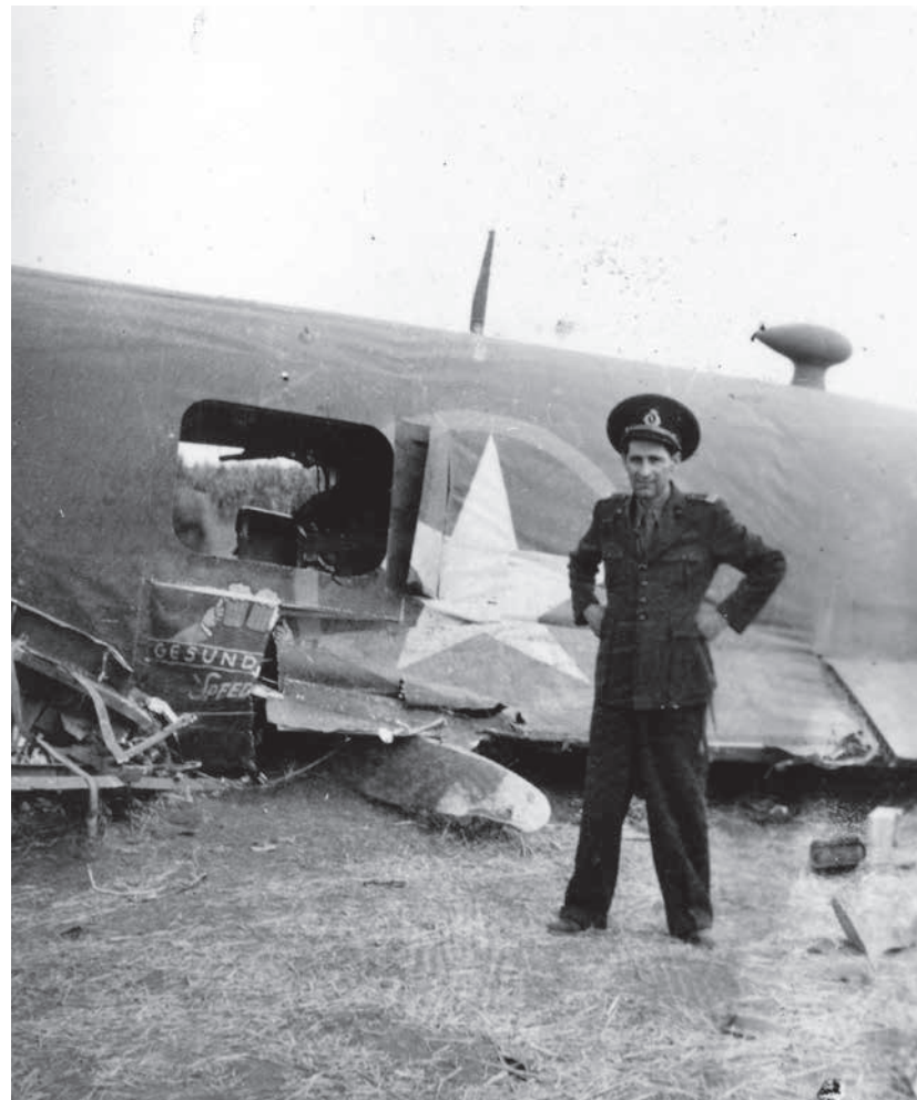
A Romanian sergeant major from the sanitary service. stands proudly near the right waist section of the crash-landed "Brewery Wagon." This picture reveals some of the terrible damage the aircraft suffered when it came to earth. Note the propeller blade sticking out below the crumpled fuselage, violently sheared off from one of the engines in the landing, which contributed to the aircraft's catastrophic damage. Some other wreckage is on the ground at the left, perhaps some of the bomb bay racks torn out of the belly of the B-24 as the weight of the wings crushed the forward part of the aircraft.
