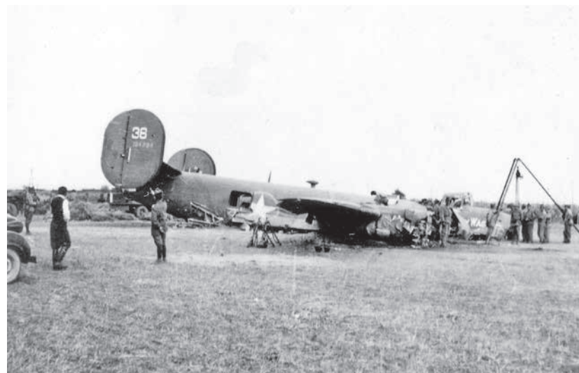
View of the right side of the wreck of B-24D "Brewery Wagon" during salvage of the wreck after the fierce Tidal Wave battle shows how crash-landed Liberator bombers often suffered extensive damage at the forward end, crushing or flattening the fuselage. Prominent is the hoist at the front end of the aircraft which appears to be used to raise the crushed nose section. The top turret abaft the grotesquely-elevated cockpit canopy frames appears to be removed. The V-shaped bit of wreckage down and left from the waist gun window could be bomb racks torn loose from the bomb bay areas crushed beneath the wings. Two rifle stacks for Romanian soldiers working at the site are seen on the ground with their "teepee" frame look, below the star on the fuselage.
